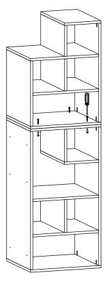
The final step would be to bolt the two components together.
