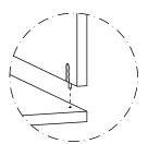
The cabienos must be align with a receiving hole
